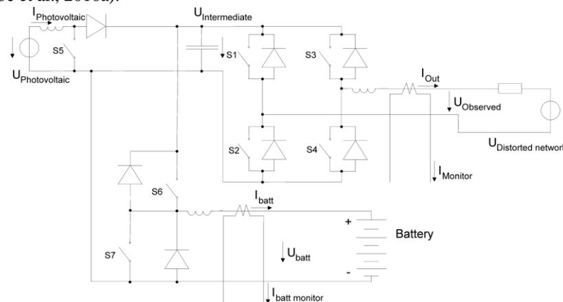
Figure 1: Grid Tie Inverter model
