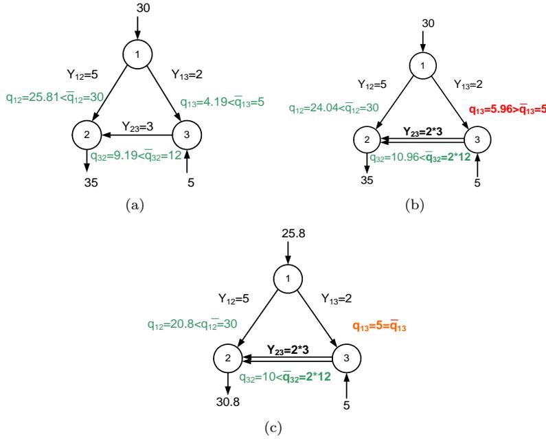
**Fig. 1** Power flow on a simple 3-node network. If we double the connection between 2 and 3, line 1-3 gets overloaded.  $Y$  denotes the line admittances.  $q_{ij}$  denotes the actual power flow on edge  $i, j$  while  $\bar{q}_{ij}$  denotes the maximum transmission capacity.
