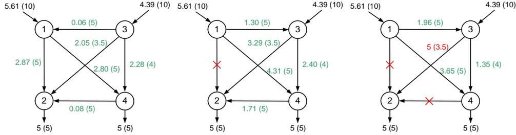
**Fig. 3** Basic (safe) operation of the 4 node network without failures, flows without rescheduling in the case of the failure of line 1-2, and in the case of the failure of line 1-2 and 2-4: The first failure does not lead to line overload, but without rescheduling the second failure causes the overload of line 2-3.
