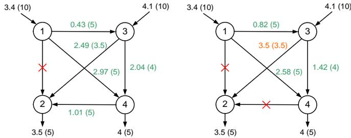
**Fig. 4** Rescheduling of the network after the failure of line 1-2: The second failure of line 2-4 does not overload the remaining lines. Line 2-3 operating on the edge of his capacity shows, that the rescheduling of generators and the curtailment of loads was justified.
