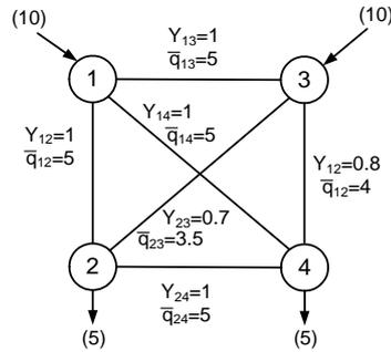
**Fig. 2** The basic structure and parameters of the 4-node network.  $Y_{ij}$  corresponds to the admittance value of the line between  $i$  and  $j$ , while  $\bar{q}_{ij}$  denotes the value of the maximal possible energy transfer on the corresponding line (power transmission capacity). The numbers in parentheses at the nodes correspond to maximal generating capacity and desired consumption.
