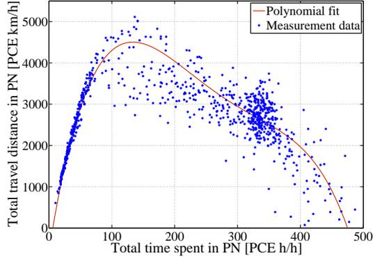
Figure 2: Fundamental diagram of the protected network
